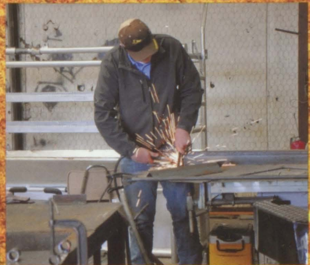
Judd Crecelius uses the cutting torch to blow out a piece of metal.
