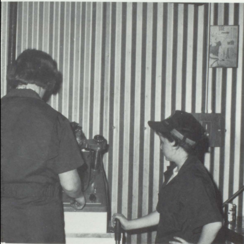
Katherine Briggs looks on as Gerald Treas assists her in installing points, using a distributor stroboscope.
